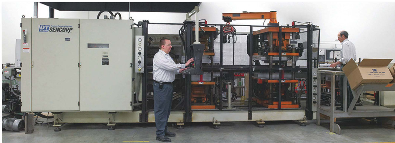
The multi-pocketed clamshell packages are thermoformed at a rate of approximately 3,000/hr.
