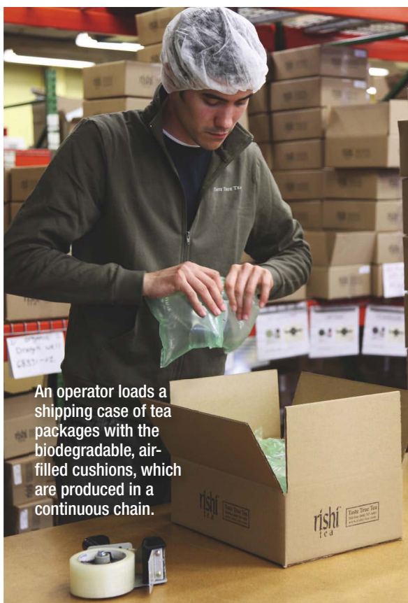
Paperboard cartons and metal tins can be easily loaded into a shipping case and blocked and braced with the biodegradable cushions, which Rishi says provide sufficient protection for its products and help lower incidences of damage.
