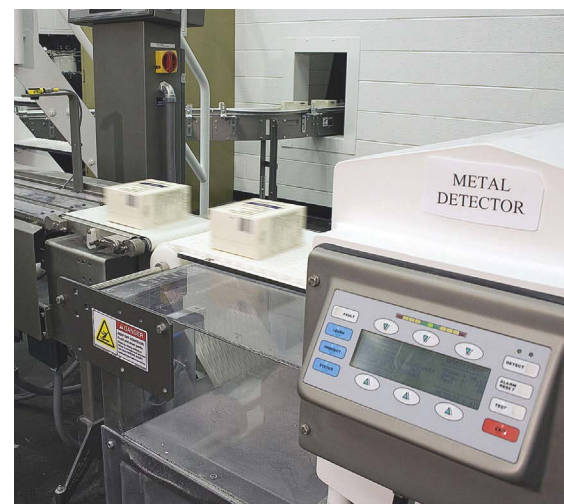
A metal detector is used on an OTC topical powder line in Royston that runs nonmetal and nonfoil pouches; other packaging lines that run metallic pouches are equipped with x-ray detection systems.
