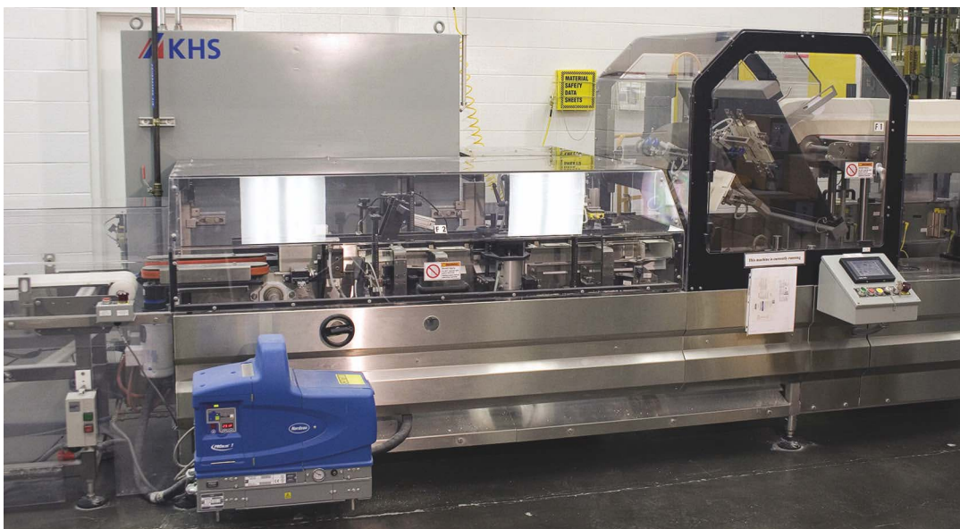
Above, in PTI's Union, MO, production facility, an auger powder filler integrated with a capper runs tall personal-care powder bottles. Top right, a pouching system in the Royston operation handles effervescent tablets with ease. PTI's production lines can generate tablet packages at speeds up to 4,000 tablets/min. Right, topical powders are pouched and cartoned on a line featuring a speedy horizontal form/fill/seal machine.
