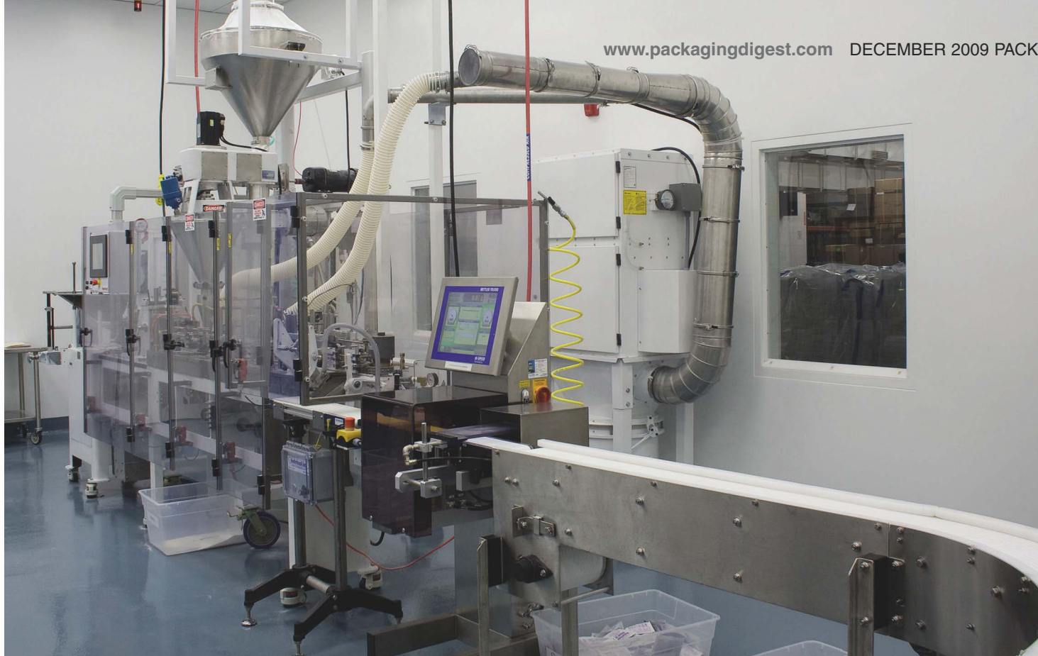
Pharma Tech Industries' pouch filling operation in Royston, GA, above, includes a clean room equipped with a horizontal form/fill pouch machine for prescription unit-dose ingestible powders. An in-line x-ray system, below left, is also included in one of the clean rooms in Royston.
