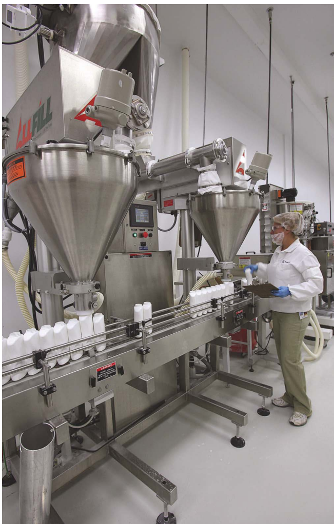
Above, in PTI's Union, MO, production facility, an auger powder filler integrated with a capper runs tall personal-care powder bottles. Top right, a pouching system in the Royston operation handles effervescent tablets with ease. PTI's production lines can generate tablet packages at speeds up to 4,000 tablets/min. Right, topical powders are pouched and cartoned on a line featuring a speedy horizontal form/fill/seal machine.
